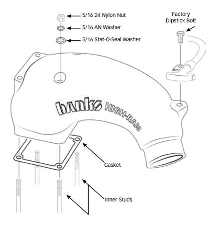
Figure 4. Exploded view of the Monster-Ram assembly
